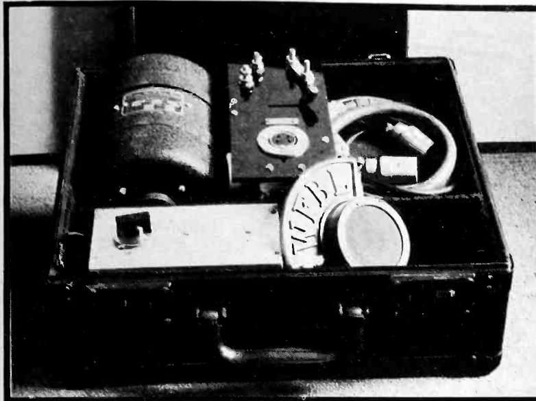
View of the power-supply case which contains also the microphone, cables and antenna tuning unit
