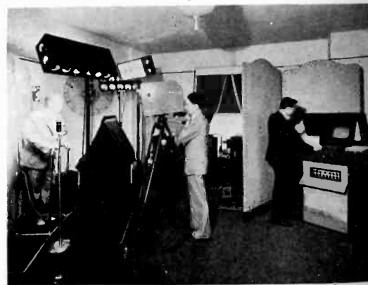
Temporary television studio, recently set up in the Ambassador Hotel at Atlantic City, to demonstrate two-way high-definition television. The viewer watches the image of a friend on another floor of the hotel in the receiver before him, while the television camera picks up his image from a similar receiver
